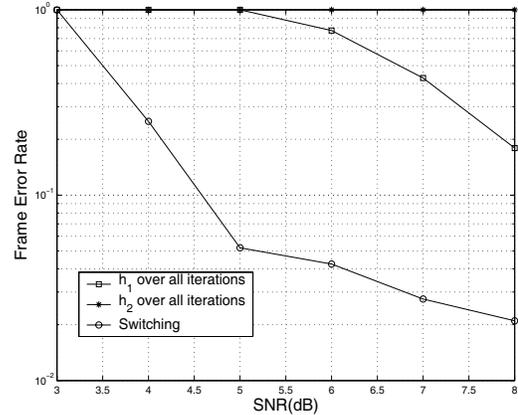
Fig. 6. FER measurement for channel B with BPSK.
