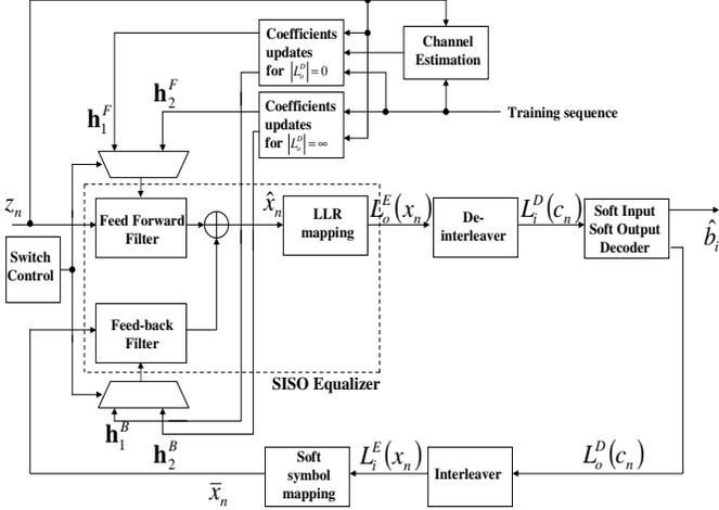
Fig. 2. A switching linear turbo-equalizer block diagram.
