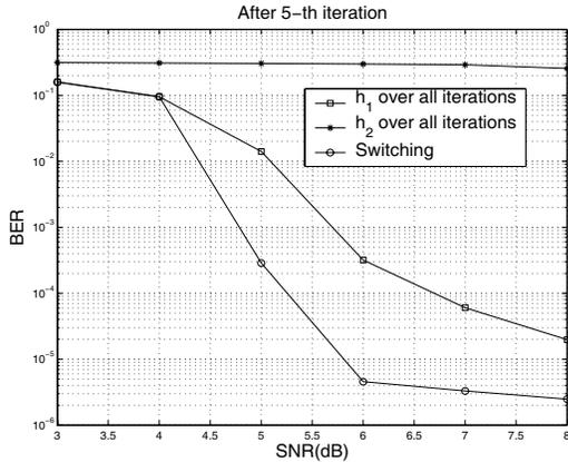
Fig. 5. BER measurement for channel B with BPSK.
