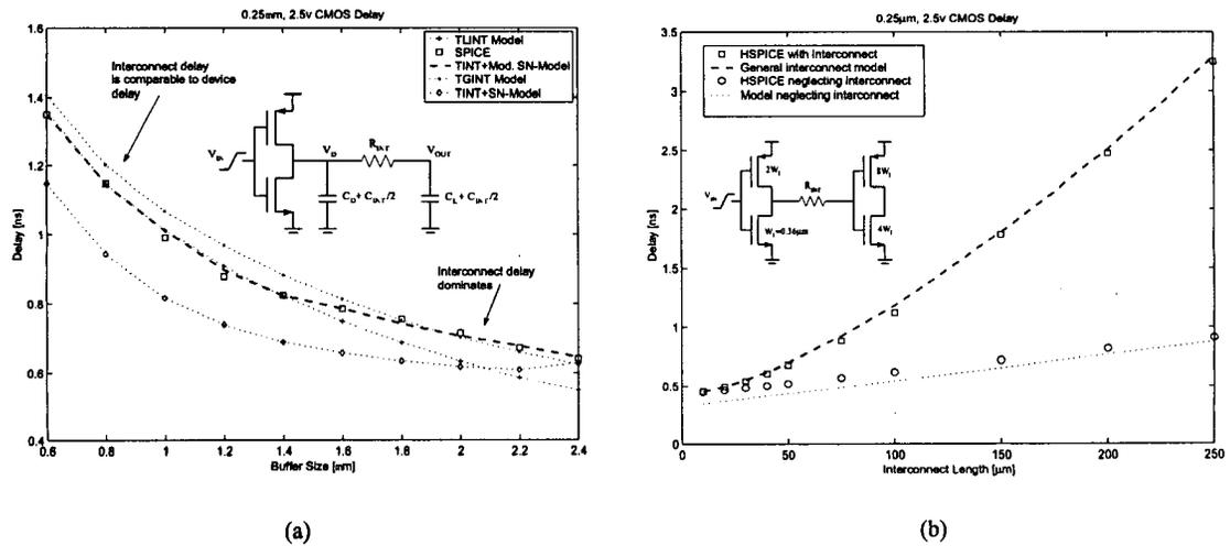
Figure 3: Inverter delay with wire resistance for (a) different buffer sizes and (b) wire lengths.
