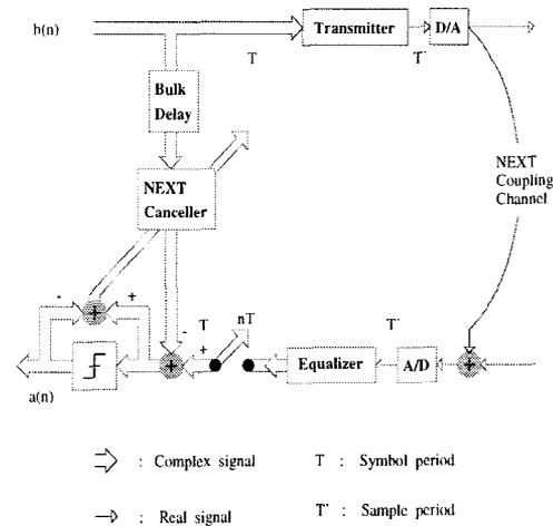
Fig 4. Block Diagram of the ATM-LAN Transceiver
