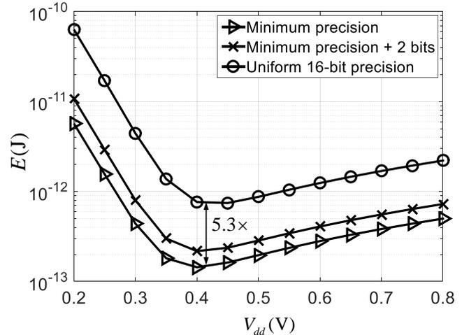
**Fig. 3:** Energy savings using minimum precision ( $B_F = 6$ ,  $B_X = 5$ ,  $B_W = 10$ ) for  $p_m < 0.01$ , compared to 2 b higher precision ( $B_F = 8$ ,  $B_X = 7$ ,  $B_W = 12$ ) and uniform precision assignment of 16 b ( $B_F = 16$ ,  $B_X = 16$ ,  $B_W = 16$ ).
