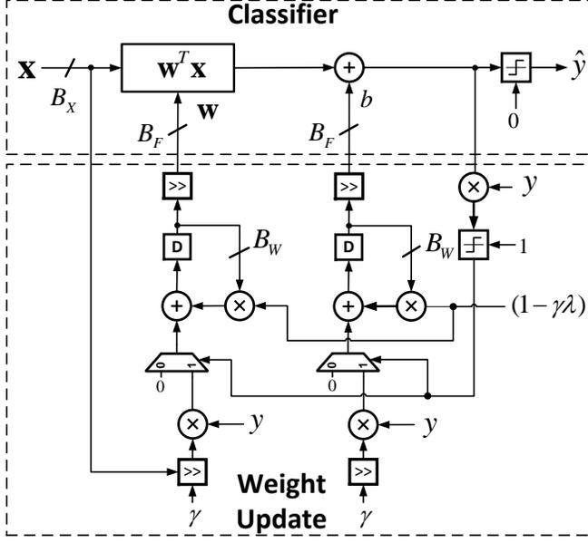
**Fig. 1:** SVM-SGD algorithm's architecture showing the precision per dimension.
