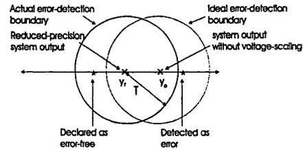
Figure 5: Error-detection boundary of reduced system
