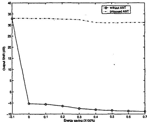
Figure 9: Energy savings vs. SNR plot of the proposed ANT scheme in  $0.25 \mu\text{m}$  CMOS technology with  $\alpha = 1.2$
