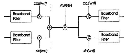
Figure 7: Receiver baseband filtering by proposed RPR based ANT scheme
