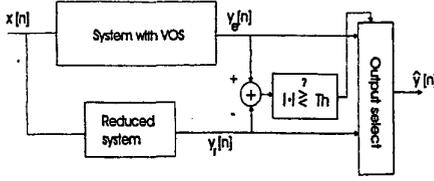
Figure 1: Overview of proposed algorithmic noise tolerance (ANT) scheme using reduced precision redundancy
