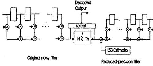
Figure 2: Proposed ANT scheme using reduced precision redundancy
