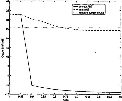
Figure 3: Performance of proposed algorithmic noise tolerance (ANT) system employing reduced precision redundancy
