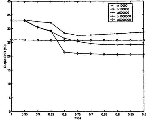
Figure 4: Performance of ANT system for the threshold variation
