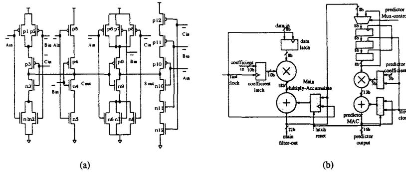
Figure 2: The soft DSP implementation: (a) schematic diagram of the 24 transistor full-adder, and (b) the filter architecture.
