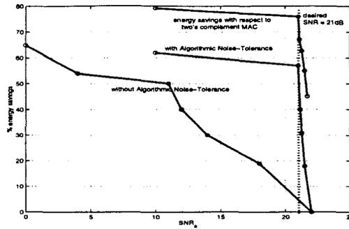
Figure 4: energy-dissipation vs. algorithmic performance for the soft DSP filter.
