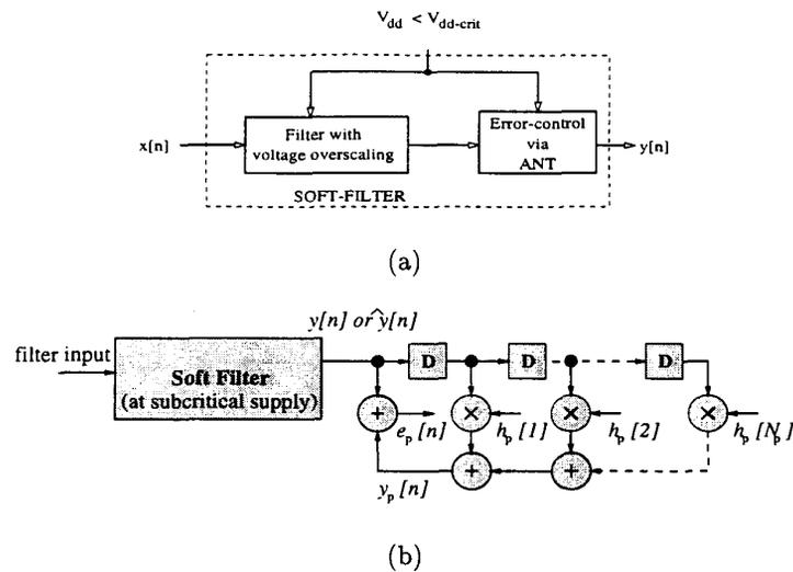
Figure 1: The soft DSP framework: (a) voltage overscaling, and (b) prediction-based algorithmic noise-tolerance scheme.
