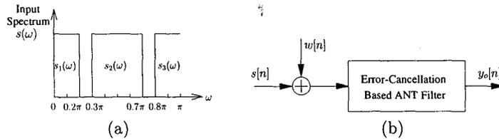
Figure 4: Simulation setup: (a) input signal spectrum and (b) lowpass filtering via the proposed ANT scheme.
