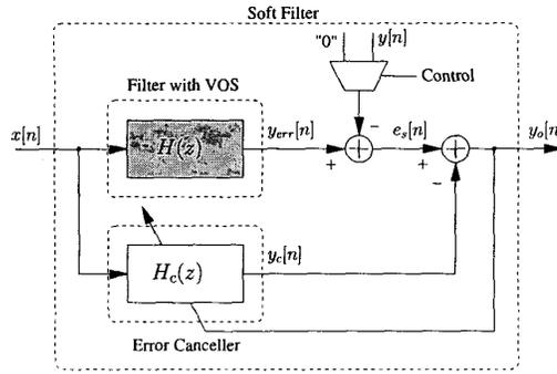
Figure 2: The proposed ANT scheme based on adaptive error-cancellation.
