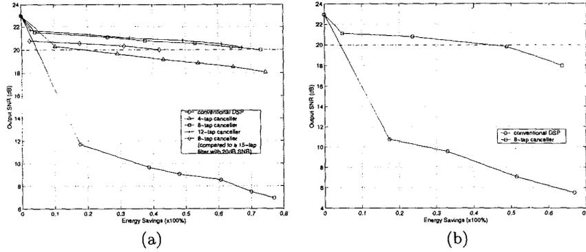
Figure 5: Performance of the proposed ANT scheme: (a) serial and (b) pipelined architecture.
