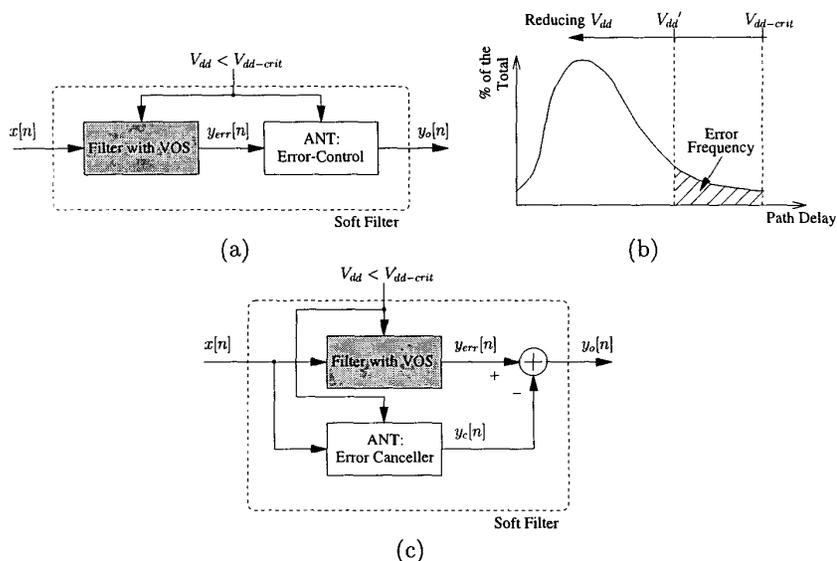
Figure 1: Soft DSP framework: (a) the error-control scheme in [5], (b) typical path delay distribution of a ripple-carry adder and (c) the proposed error-cancellation scheme.
