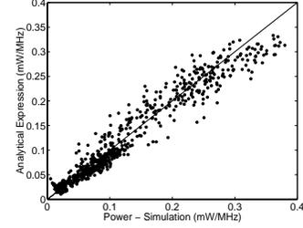
Figure 10: Validation of analytical expression for multiplier power dissipation
