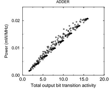
Figure 7: Variation of power with total output bit transition activity for adder
