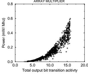
Figure 9: Variation of power with total output bit transition activity for multiplier
