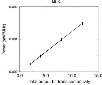
Figure 6: Variation of power with total output bit transition activity for a multiplexer
