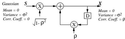
Figure 4: Signal generation model
