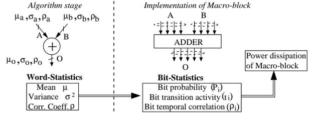
Figure 2: Relationship between signal statistics and power dissipation
