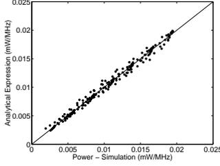
Figure 8: Validation of analytical expression for adder power dissipation
